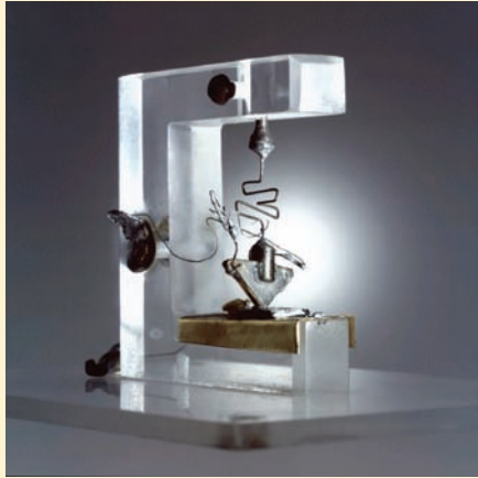
■ FIGURE 17.27 Photograph of the first demonstrated bipolar junction transistor (“bjt”). Lucent Technologies Inc/Bell Labs
