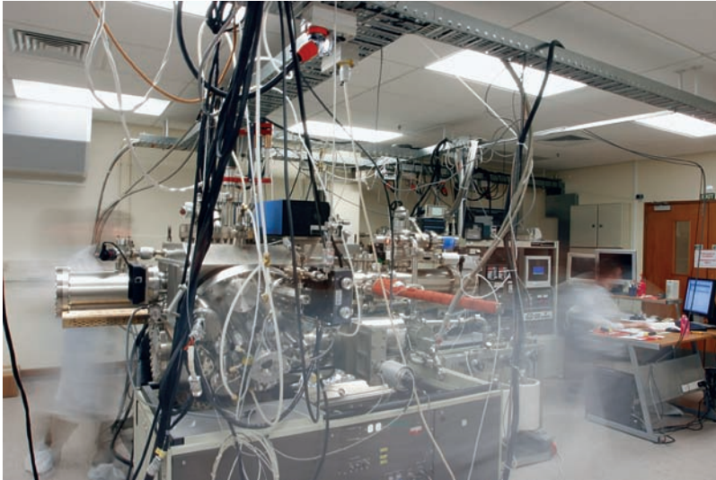
A molecular beam epitaxy crystal growth facility. The equations governing its operation closely resemble those used to describe simple linear circuits.
