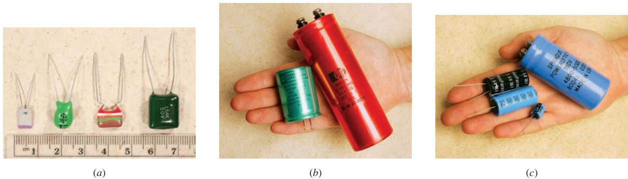
■ FIGURE 7.2 Several examples of commercially available capacitors. (a) Left to right: 270 pF ceramic, 20 \mu\text{F} tantalum, 15 nF polyester, 150 nF polyester. (b) Left: 2000 \mu\text{F} 40 VDC rated electrolytic, 25,000 \mu\text{F} 35 VDC rated electrolytic. (c) Clockwise from smallest: 100 \mu\text{F} 63 VDC rated electrolytic, 2200 \mu\text{F} 50 VDC rated electrolytic, 55 F 2.5 VDC rated electrolytic, and 4800 \mu\text{F} 50 VDC rated electrolytic. Note that generally speaking larger capacitance values require larger packages, with one notable exception above. What was the tradeoff in that case?
